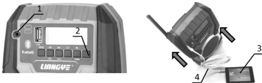
Auxiliary input socket (AUX IN) 2. Power switch button 3. USB device 4. AUX cable
